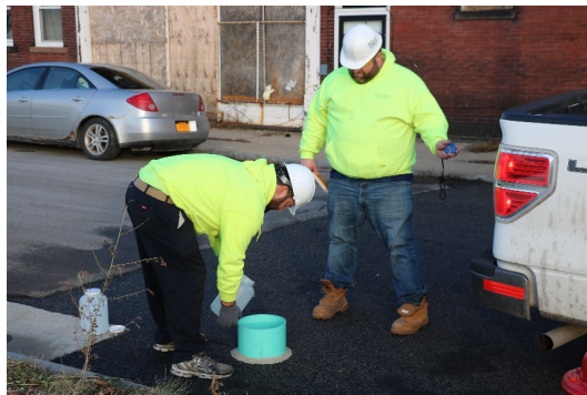
Infiltration testing of porous asphalt
